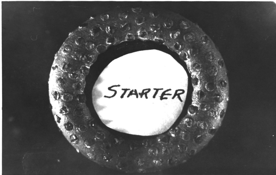
Figure 34. Starter bit used to collar holes.
