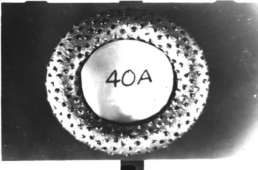
Figure 19. Bit 40a before drilling.
