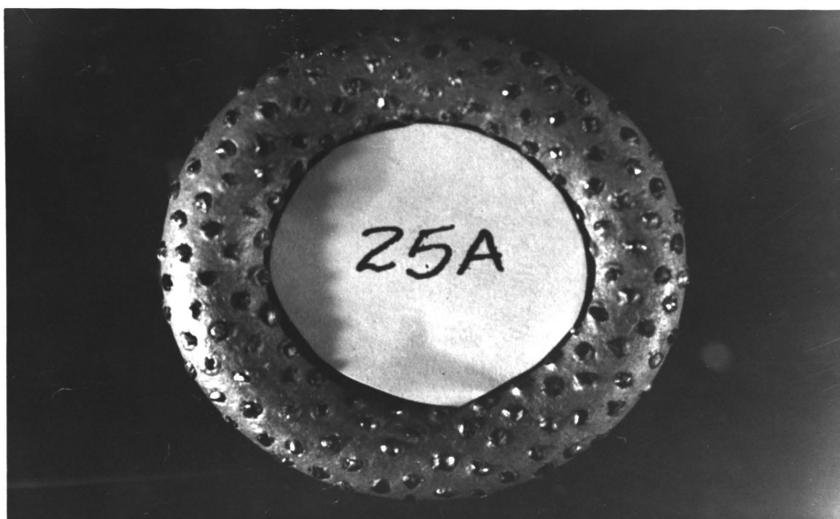
Figure 16. Bit 25a after drilling.
